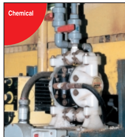
This ARO 666057-444 pumps magnesium sulfate
